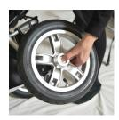
Push small axle through rear wheel. Locate in axle unit and push chrome cap until axle firmly locked. Remove rear wheels by pushing in chrome cap and pull unit out of rear frame.
