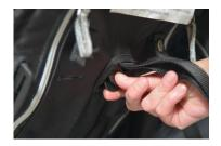
To move backrest to upright position squeeze clip and pull strap whilst pushing backrest to desired position.
